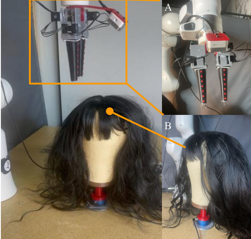
Figure 8: Experimental setup for evaluating the proposed MOE in interaction with a force-sensitized mannequin head. A: Two-fingered MOE soft manipulator with an RGBD camera. B: Mannequin head with a wig and 6-axis force sensor at its base.
