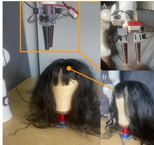
Figure 3: Experimental setup for evaluating the proposed MOE in interaction with a force-sensorized mannequin head. A: Two-fingered MOE soft manipulator with an RGBD camera. B: Mannequin head with a wig and 6-axis force sensor at its base.
