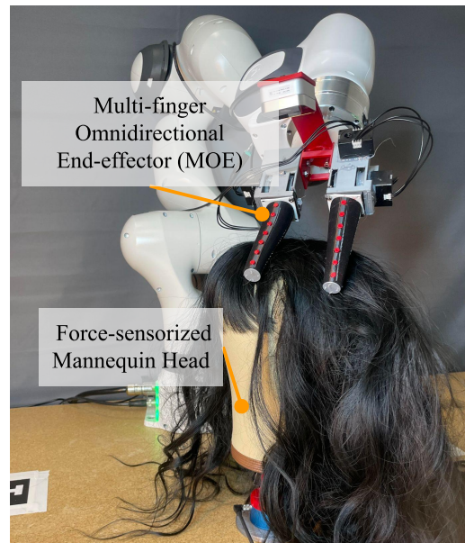
Figure 1: Proposed Multi-finger Omnidirectional End-effector (MOE) and a force-sensorized mannequin head in contact. Contact between the head and MOE deforms MOE’s fingers, resulting in safer interaction forces.
